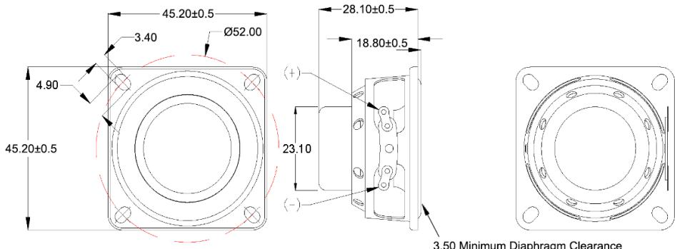
General tolerance = ±0.5 mm and all measurements in mm unless otherwise noted.
