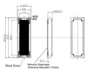
General tolerance =  $\pm 0.2$  mm and all measurements in mm unless otherwise noted.
