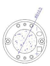
General tolerance =  $\pm 0.2$  mm and all measurements in mm unless otherwise noted.
