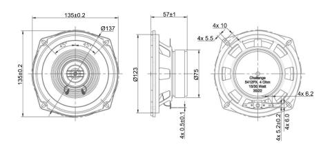
General tolerance =  $\pm 0.3$  mm and all measurements in mm unless otherwise noted.
