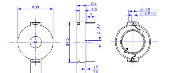
(Unit:mm, Tolerance: +/-0.3mm)
