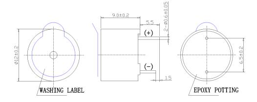
General tolerance = ±0.5 mm and all measurements in mm unless otherwise noted.
