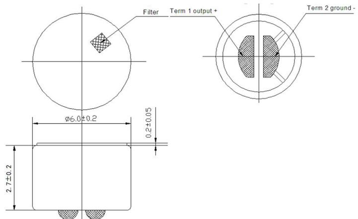
General tolerance =  $\pm 0.2$  mm and all measurements in mm unless otherwise noted.
