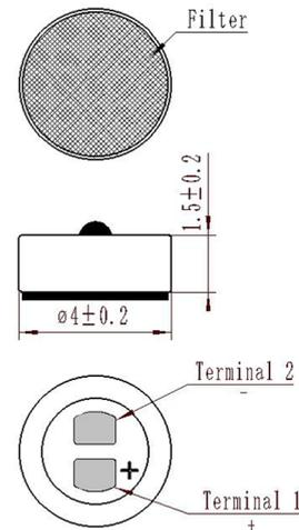
General tolerance = ±0.2 mm and all measurements in mm unless otherwise noted.
