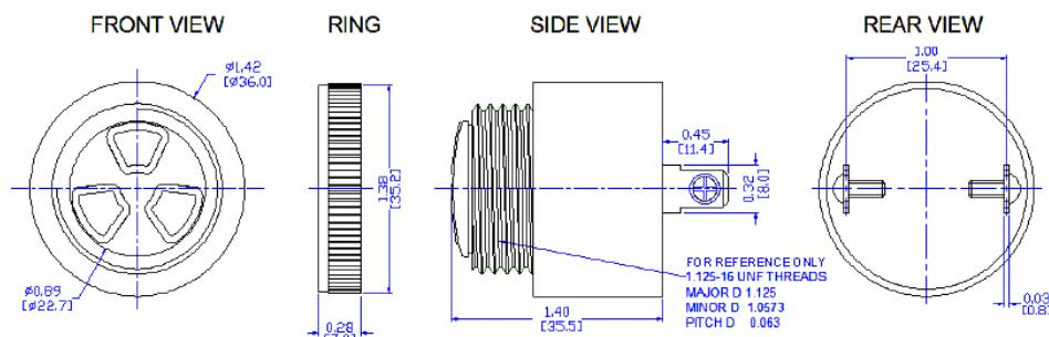
General tolerance = ±0.7 mm and all measurements in mm unless otherwise noted.
