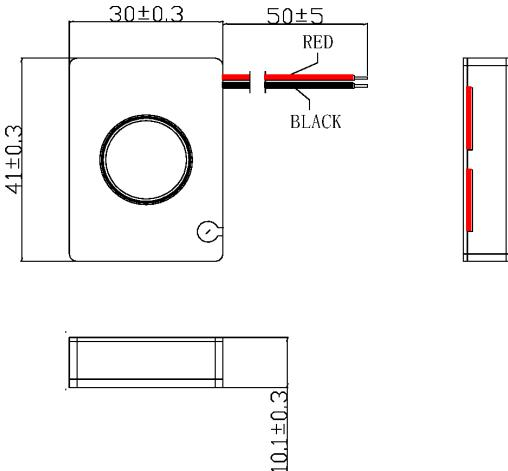
General tolerance = ±0.5 mm and all measurements in mm unless otherwise noted.
