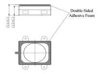
General tolerance =  $\pm \le 2$  mm:  $\pm 0.1$  mm, >2 mm:  $\pm 0.3$  mm and all measurements in mm unless otherwise noted.
